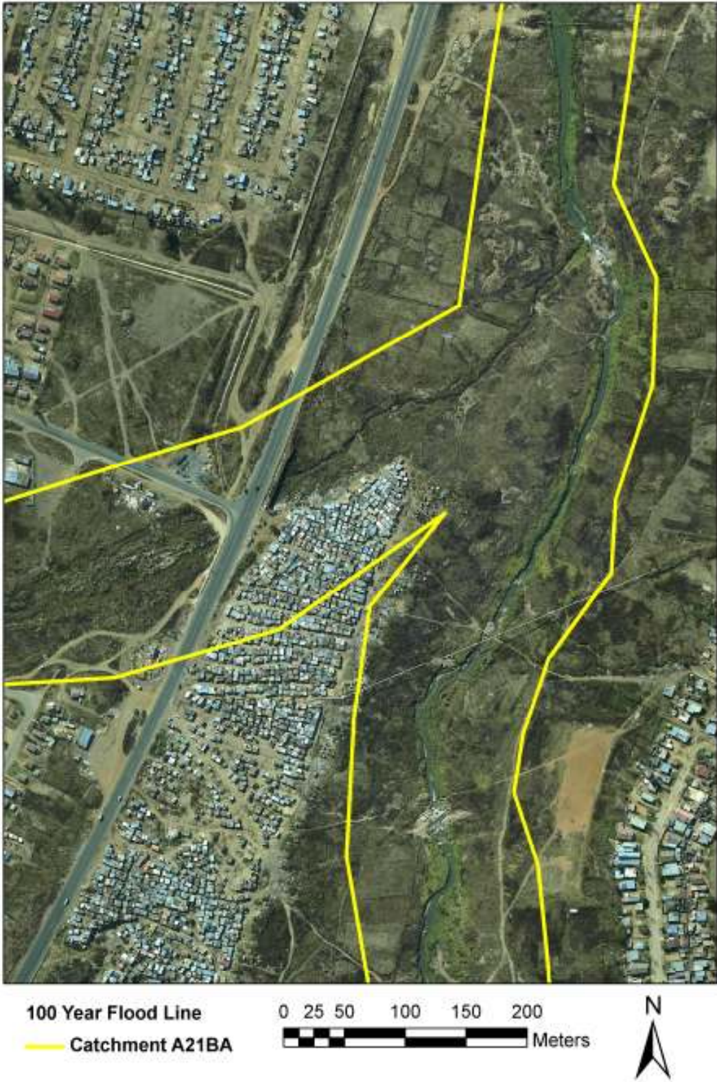
Figure 11: Potential Flood-prone Areas for Catchment A21B_A (1)
